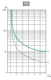
**Cold curve:** represents the performance of the relay without any previous current flow, first start.
