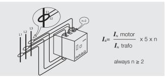
With current transformers it is always a must to pass the conductors 2 times or more through the holes of the relay.
