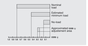
b) A slightly oversized motor for its application. The cos  $\phi$  of the motor is 0,25 when working without load.
