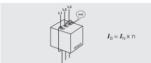
c) For motor or generator rated currents (I<sub>N</sub>) above the range of the relay, use three current transformers .../5 in combination with the C9, GL16, P19, PF16-R, G17, BG17 or GEN10 according to application.
