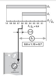
b) If the value of the  $I_{\rm B}$  of the motor without load is unknown:
