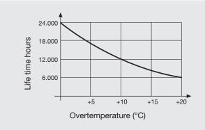
As one can see, a 10°C increase in temperature reduces the useful life of the motor by half.
