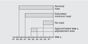
If the above mentioned  $\cos\phi$  values are unknown, the underload trip setting can be made in the following way:
